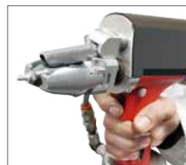
Phase 3 - Blind rivet loaded
